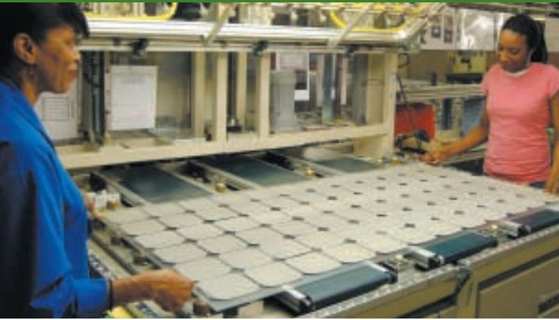
Two members of the International Brotherhood of Electrical Workers (IBEW) assemble photovoltaic modules at the Sharp Electronics plant in Memphis, where production has increased 56 percent, to 100 megawatts annually. Courtesy IBEW
